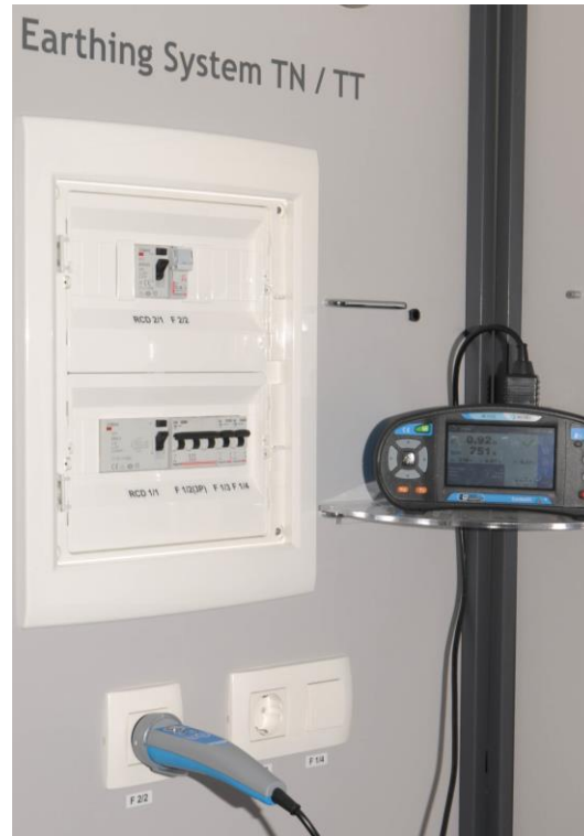
Figure 2-25: RCD measurement in the Application Trainer with the schuko commander
