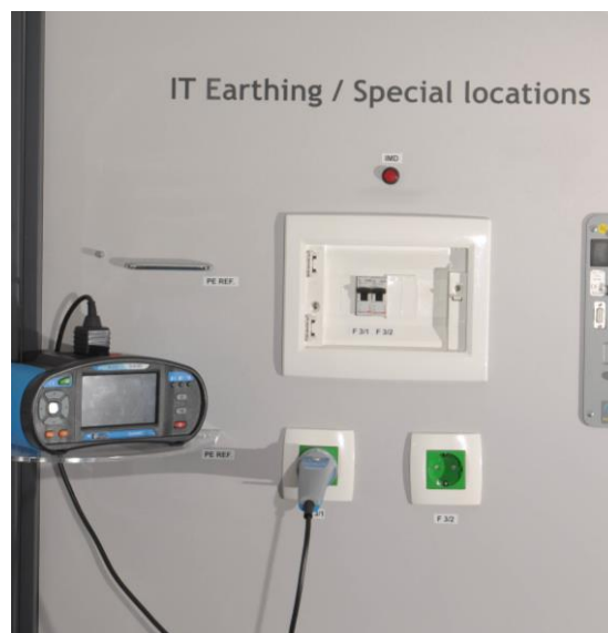
Figure 2-29: Measuring I_{SFL} and IMD in an IT system
