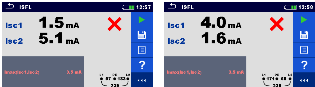
Figure 2-30: ISFL simulated errors on an IT system
