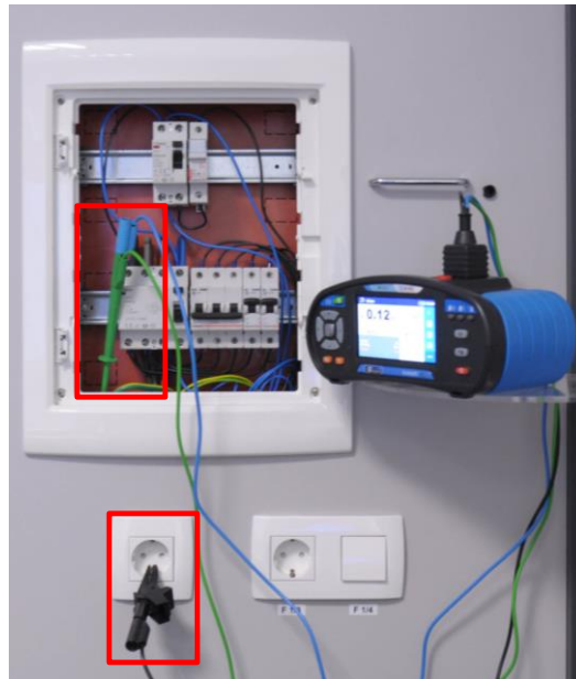
Figure 2-43: Continuity measurement between switchboard and socket
