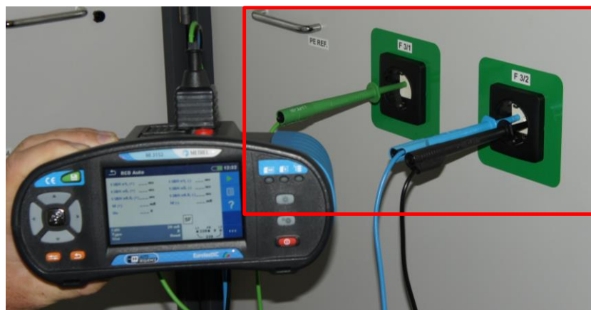
Figure 2-26: RCD measurement in an IT earthing system
